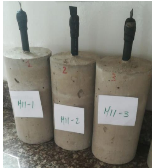
Figure 14. Corrosion test specimens
