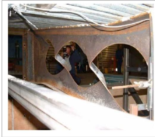
Figure 7. Web post buckling of a composite cellular beam (Nadjai et al., 2008)
