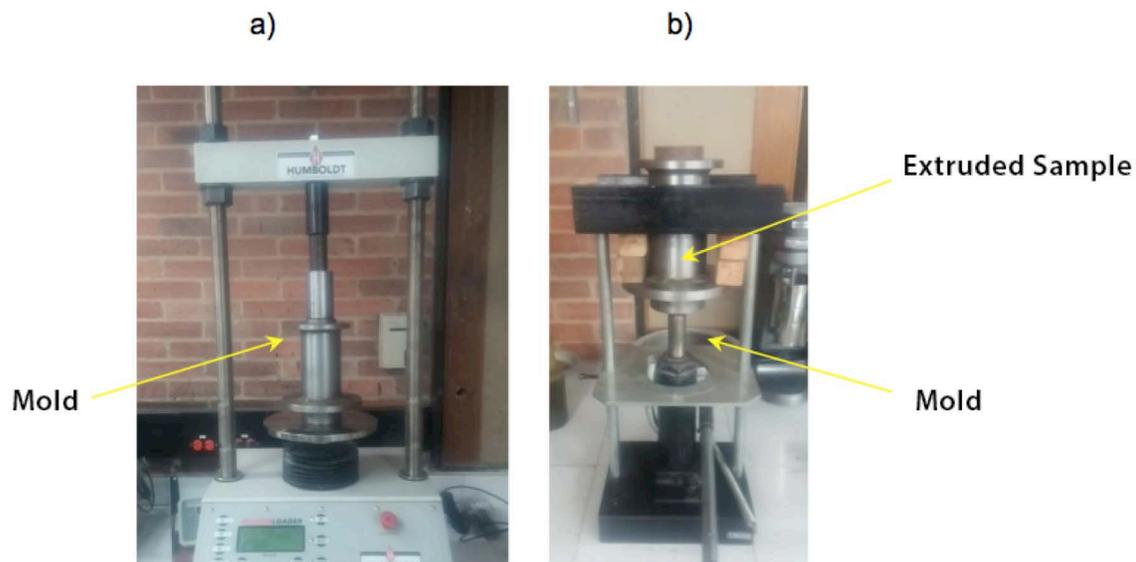
Figure 1. Compaction (a) and extrusion (b) of the specimens from the mold after the Marshall pressing
