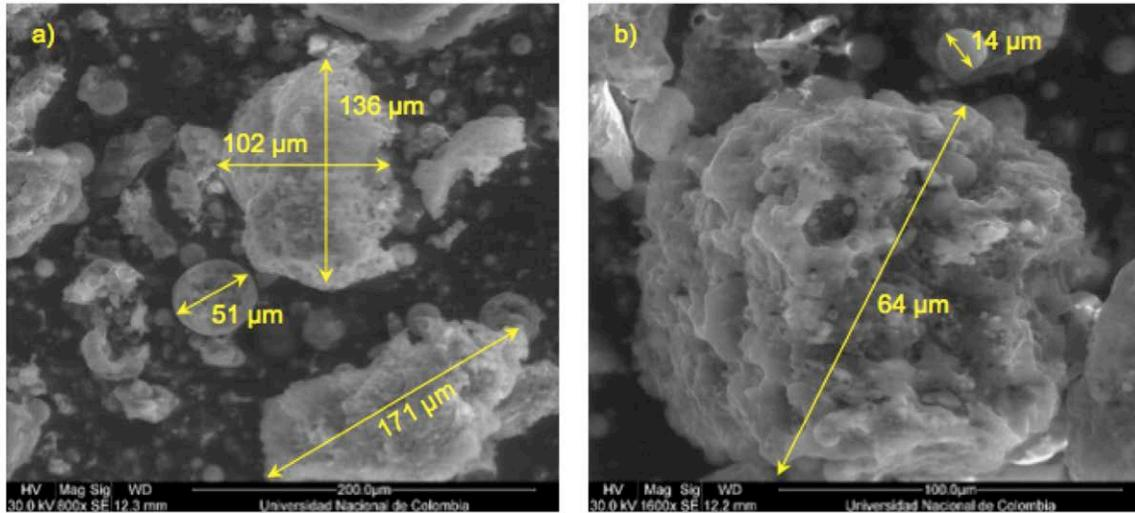
Figure 11. SEM photographs of CCR: a) 800x, b) 1600x
