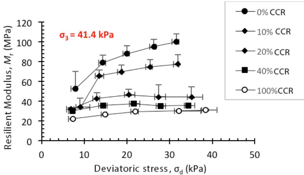
Figure 17. Variation of  $M_r$  at confinement stress of 41.4 kPa
