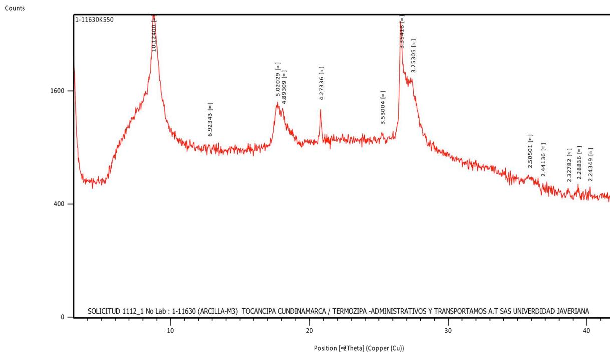
Figure 14. Diffractogram of FS at 550°C
