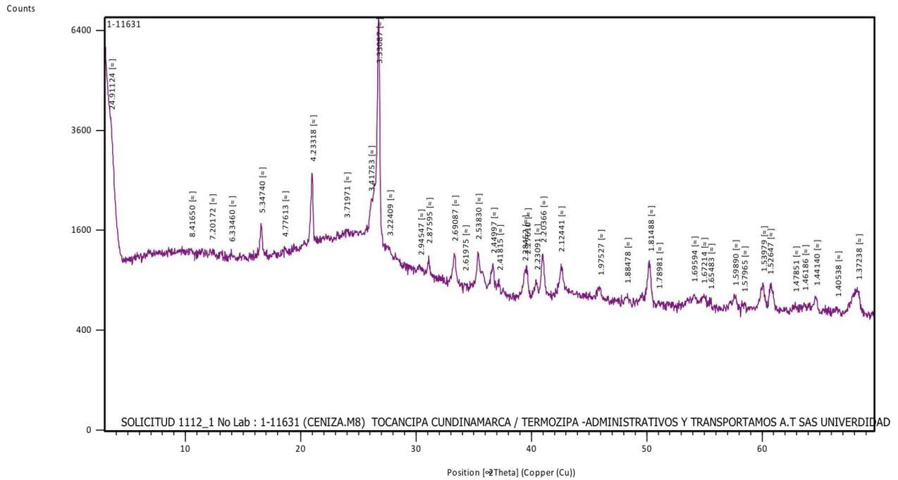
Figure 16. CCR Diffractogram
