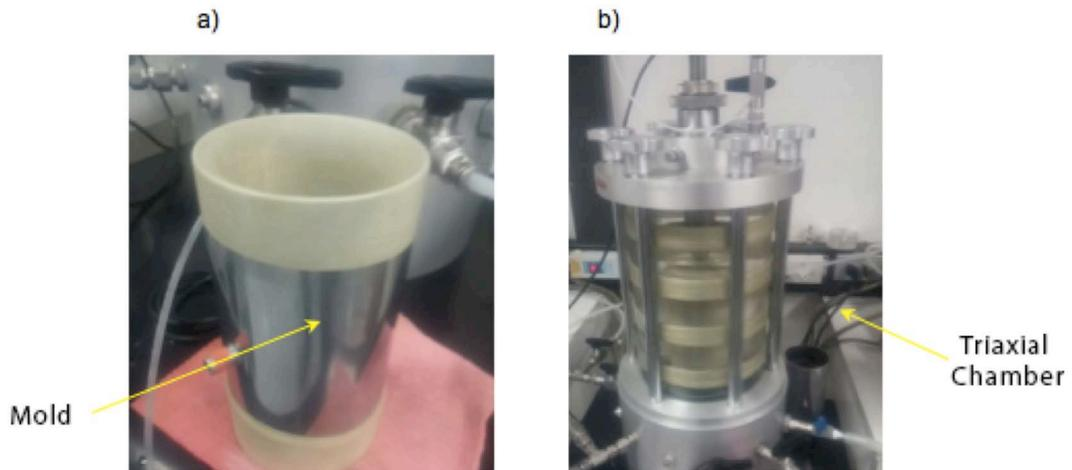
Figure 2. Assembly for measuring resilient modulus in triaxial compressive chamber
