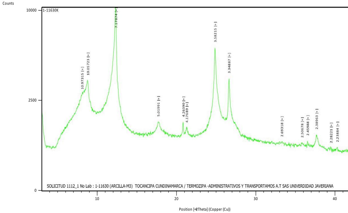
Figure 13. Diffractogram of FS with potassium (K)
