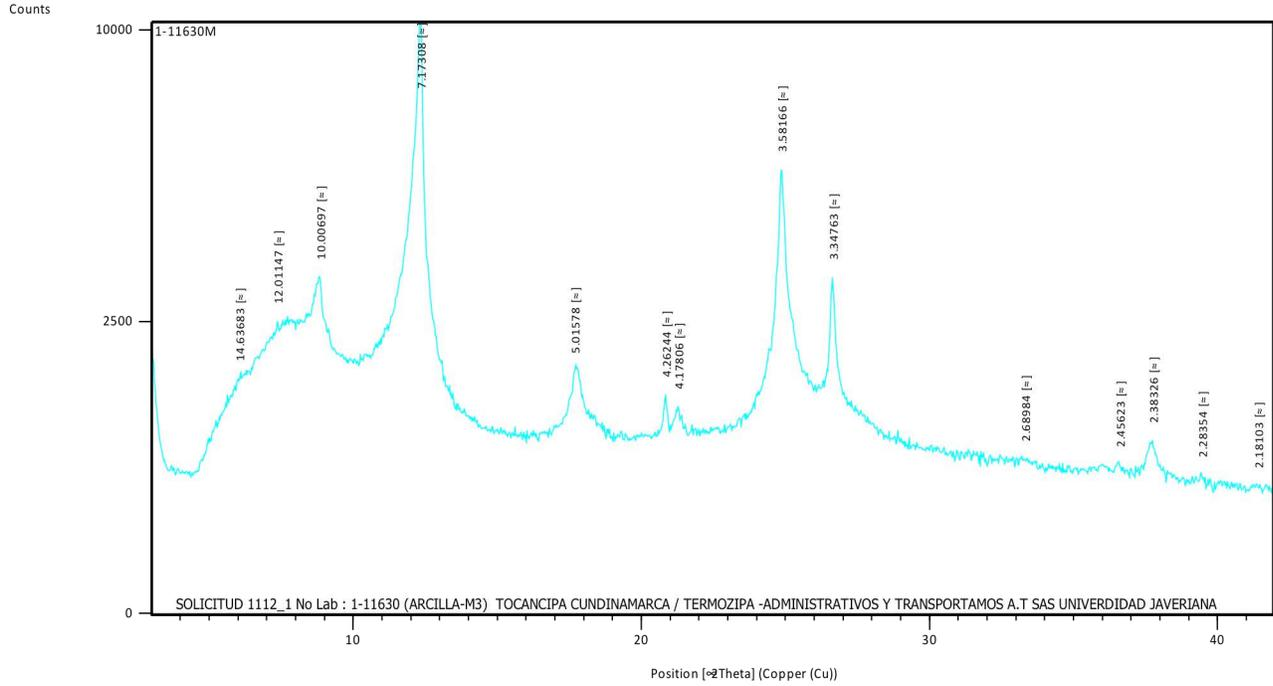
Figure 15. Diffractogram of FS with magnesium (Mg)
