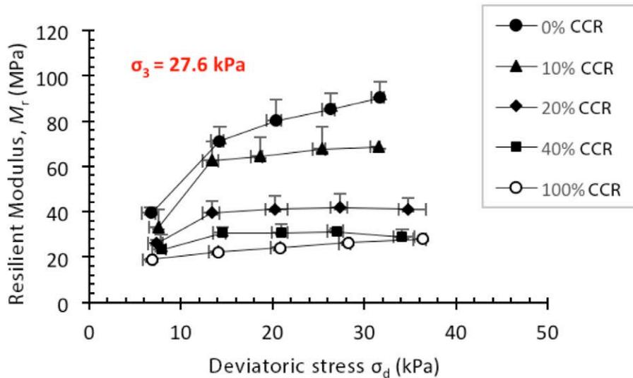
Figure 18. Variation of  $M_r$  at confinement stress of 27.6 kPa
