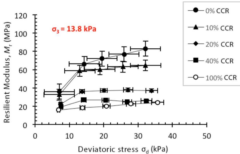
Figure 19. Variation of  $M_r$  at confinement stress of 13.8 kPa
