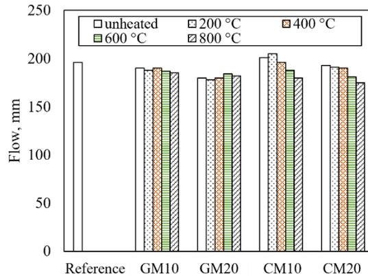
Figure 5. Flow of mortar with granite and clay powders treated at elevated temperatures.
