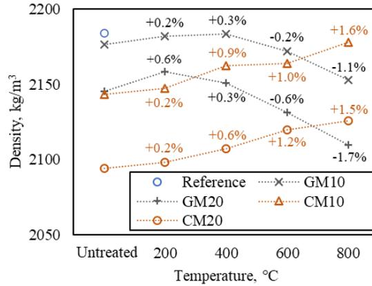
Figure 7. Density of mortar with granite and clay powders treated at elevated temperatures.
