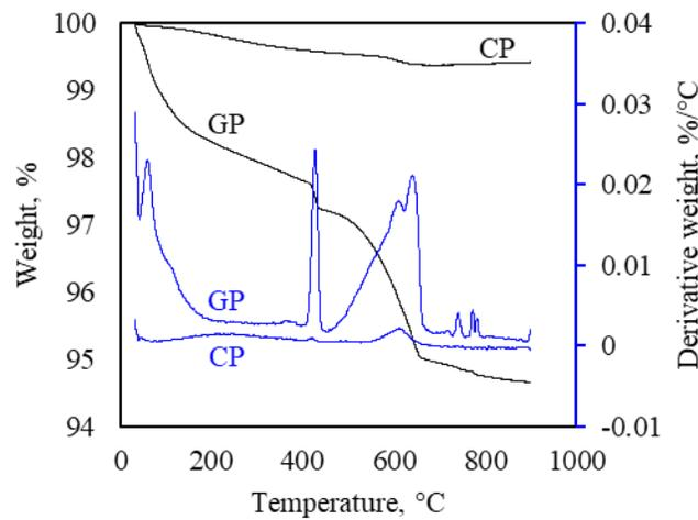
**Figure 3.** Thermogravimetric analysis of granite and clay powders.
