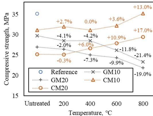
Figure 9. Compressive strength of mortar with granite and clay powders treated at elevated temperatures.
