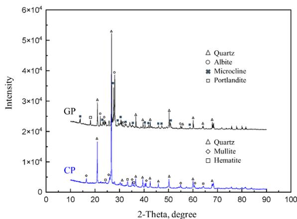
**Figure 2.** X-ray diffraction of granite and clay powders.
