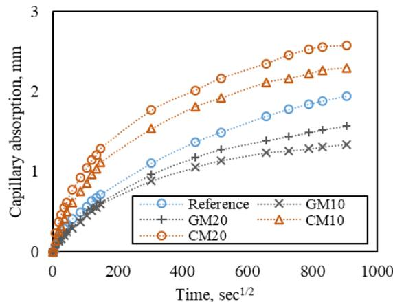
Figure 10. Capillary absorption of mortar with untreated granite and clay powders.
