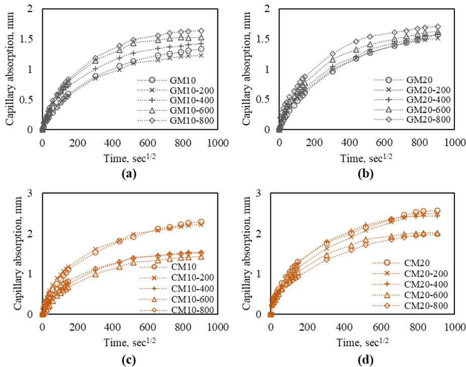
**Figure 11.** Capillary absorption of mortar with granite and clay powders treated at elevated temperatures: (a) GM10 , (b) GM20, (c) CM10, and CM20.
