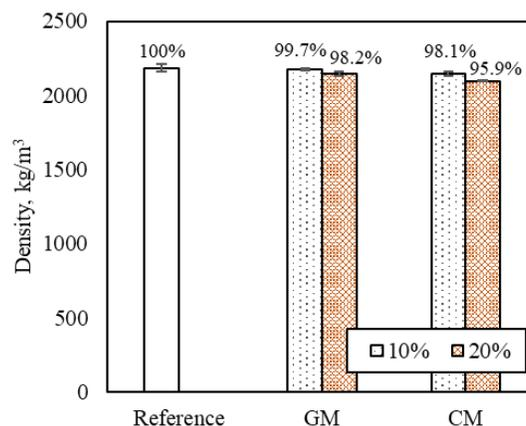
Figure 6. Density of mortar with untreated granite and clay powders.
