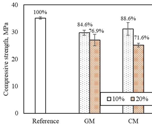
Figure 8. 28-day compressive strength of mortar with granite and clay powders.
