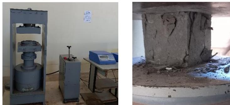
**Figure 14.** Compressive strength test.
