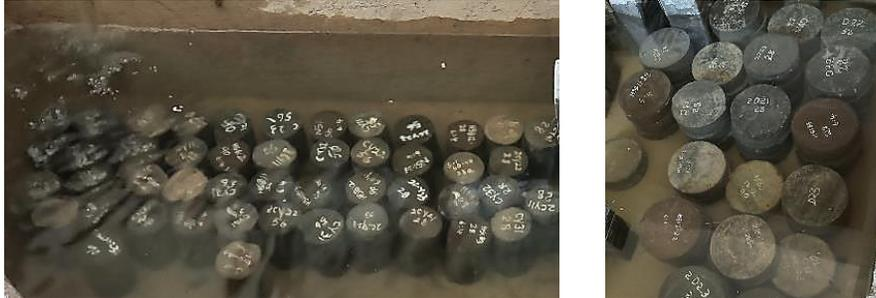
**Figure 12.** Specimens under curing.
