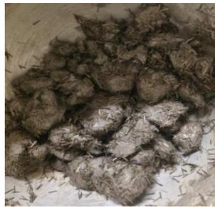
**Figure 10.** Balling effect due to further addition of basalt fiber.
