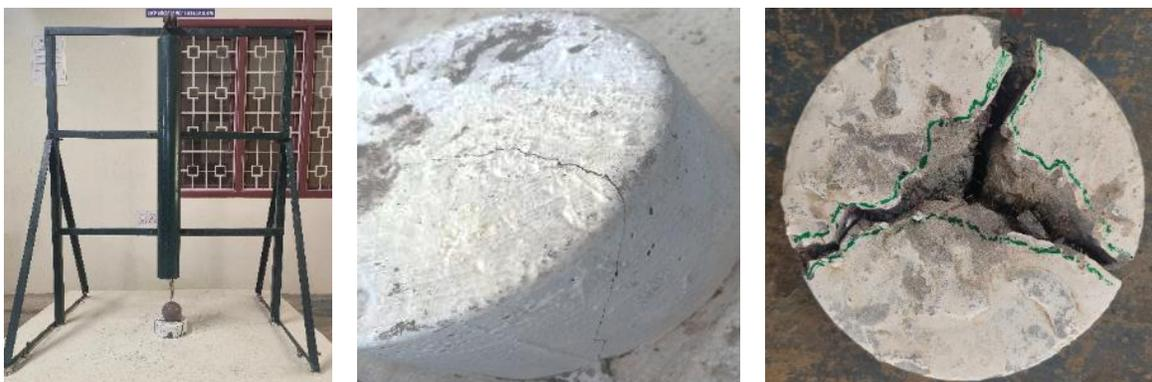
**Figure 16.** Test for impact energy resistance.
