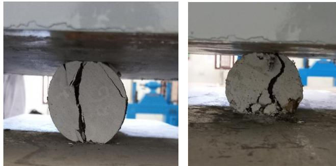
**Figure 15.** Splitting tensile strength test.
