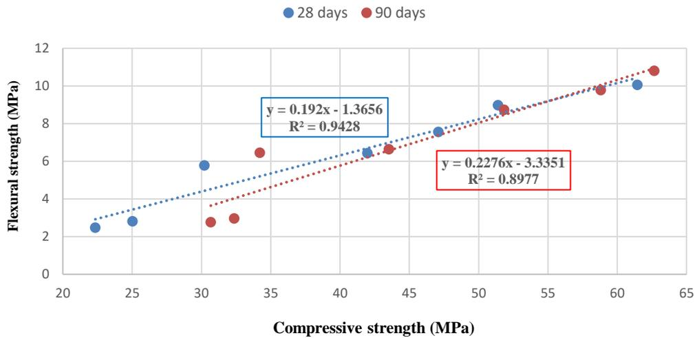
**Figure 18.** The relationship between compressive and flexural strength of concretes with a water/cement ratio of 0.4.
