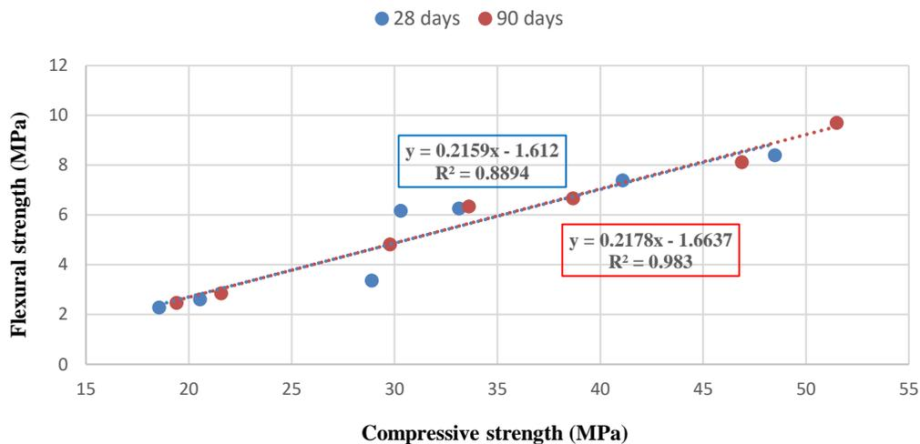
**Figure 19.** The relationship between compressive and flexural strength of concretes with a water/cement ratio of 0.5.
