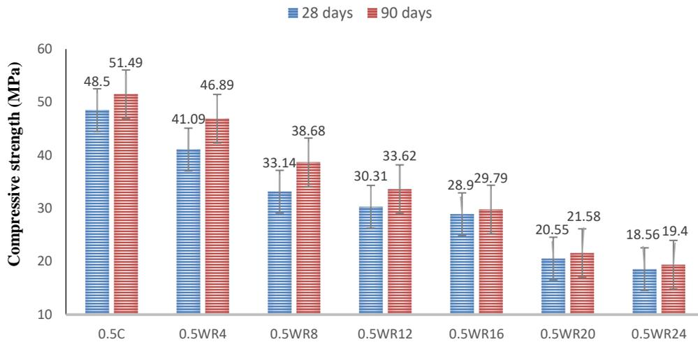
Figure 7. Effect of waste rubber substitution on compressive strength of 0.5 w/c concrete.
