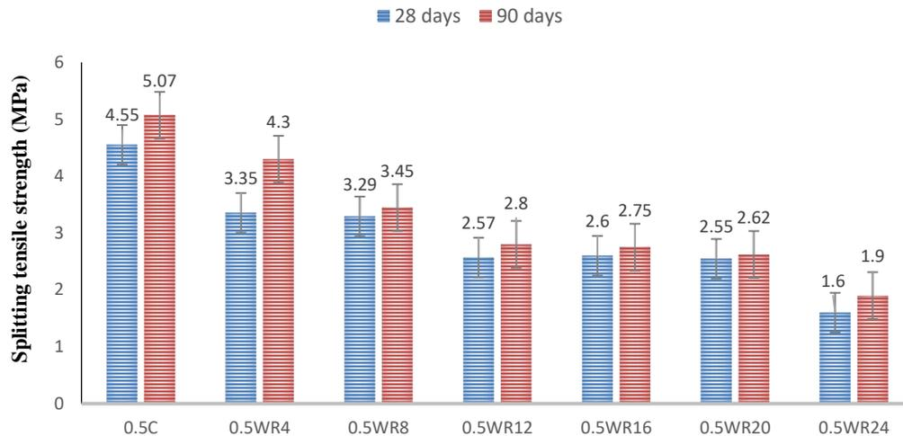
**Figure 11.** Effect of waste rubber substitution on splitting tensile strength of 0.5 w/c concrete.
