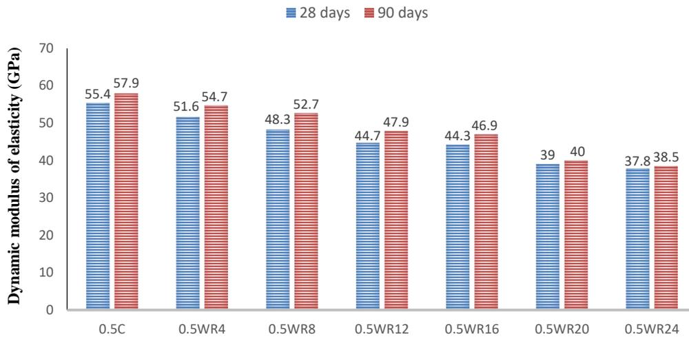
**Figure 15.** Effect of waste rubber substitution on dynamic modulus of elasticity of 0.5 w/c concrete.
