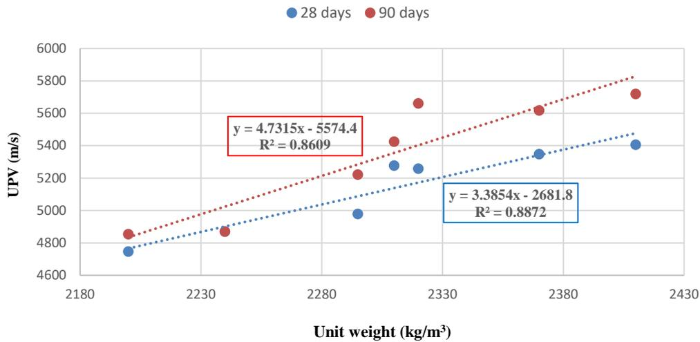
**Figure 16.** The relationship between unit weight-UPV of concretes with a water/cement ratio of 0.4.
