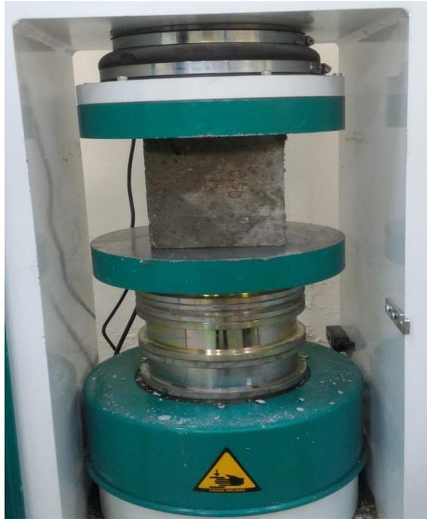
**Figure 2.** Visual of the compressive strength test.
