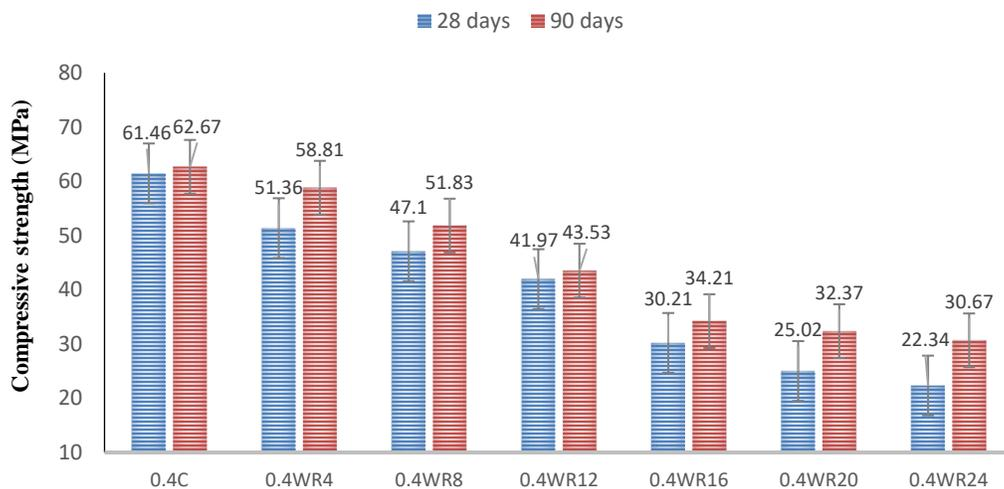
Figure 6. Effect of waste rubber substitution on compressive strength of 0.4 w/c concrete.
