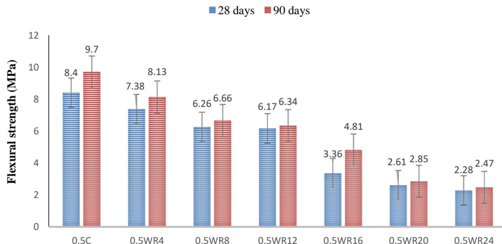
Figure 9. Effect of waste rubber substitution on flexural strength of 0.5 w/c concrete.
