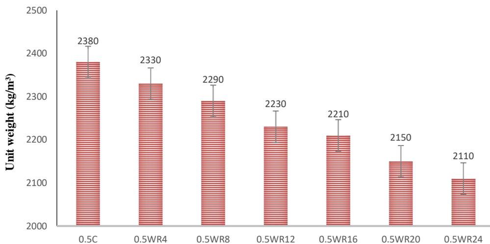
Figure 5. Effect of waste rubber substitution on unit weight of 0.5 w/c concrete.
