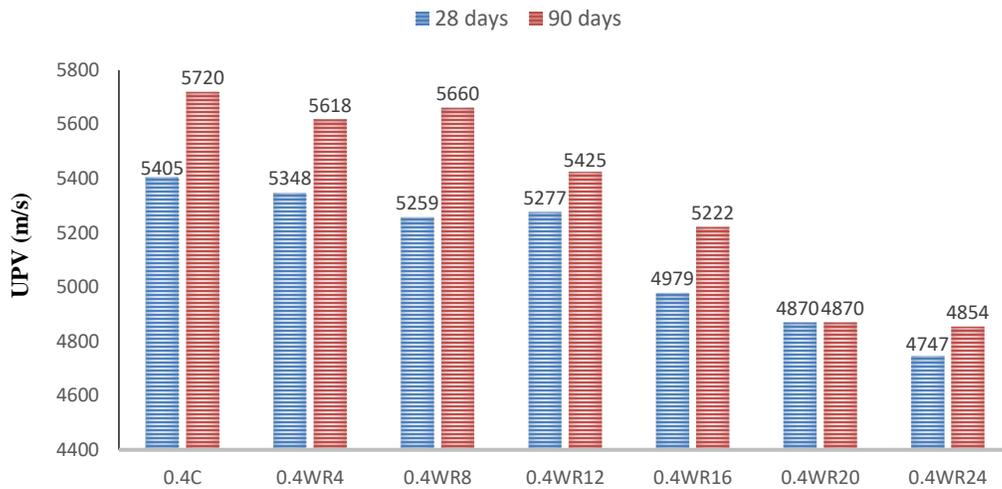
Figure 12. Effect of waste rubber substitution on UPV of 0.4 w/c concrete.
