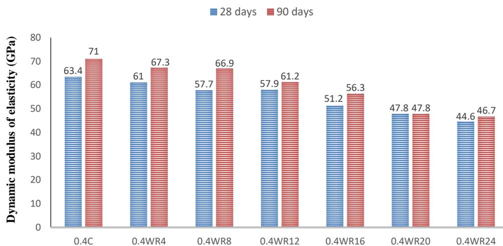
Figure 14. Effect of waste rubber substitution on dynamic modulus of elasticity of 0.4 w/c concrete.
