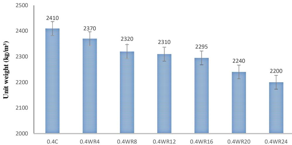
Figure 4. Effect of waste rubber substitution on unit weight of 0.4 w/c concrete.
