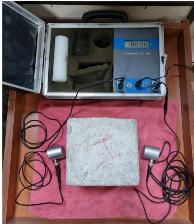
**Figure 3.** Visual of the UPV test.
