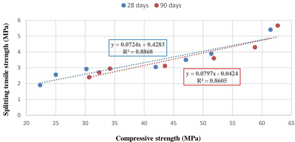
**Figure 20.** The relationship between compressive and splitting tensile strength of concretes with a water/cement ratio of 0.4.
