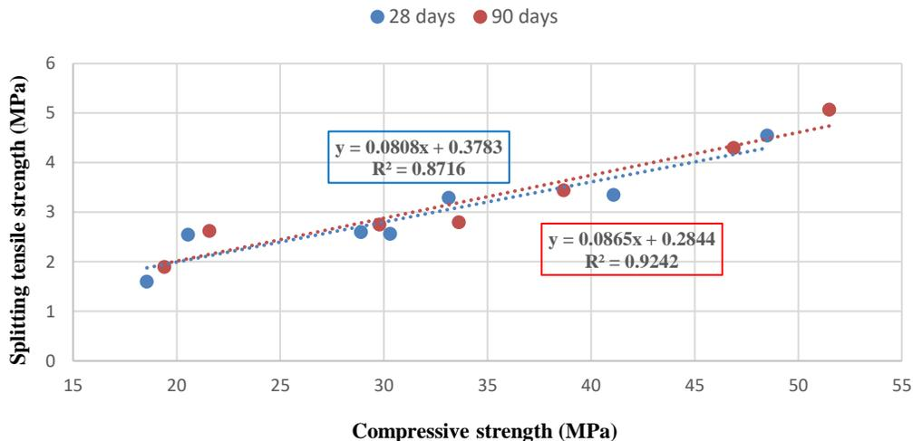
**Figure 21.** The relationship between compressive and splitting tensile strength of concretes with a water/cement ratio of 0.5.
