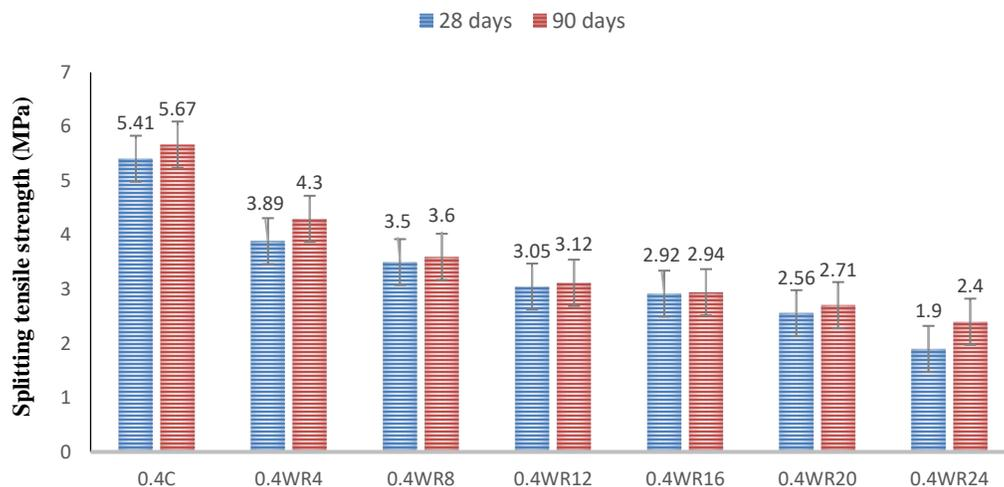
Figure 10. Effect of waste rubber substitution on splitting tensile strength of 0.4 w/c concrete.
