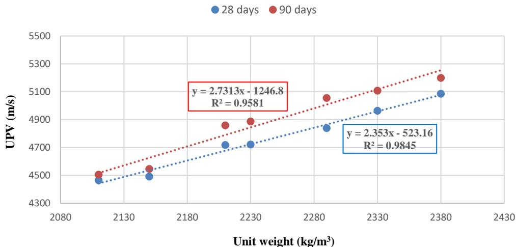
**Figure 17.** The relationship between unit weight-UPV of concretes with a water/cement ratio of 0.5.
