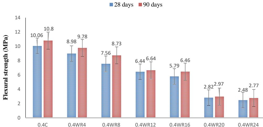
Figure 8. Effect of waste rubber substitution on flexural strength of 0.4 w/c concrete.
