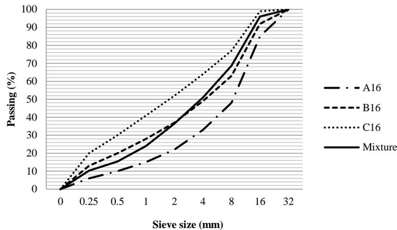
**Figure 1.** The granulometry curve of the mixture.
