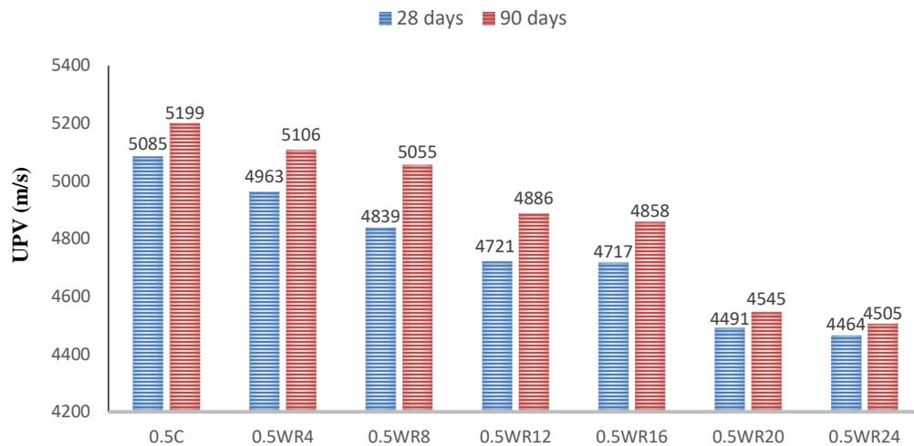
Figure 13. Effect of waste rubber substitution on UPV of 0.5 w/c concrete.
