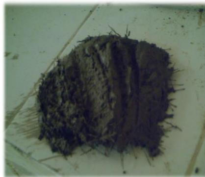
**Figure 6.** Fresh mortar mixture with crimped fiber.
