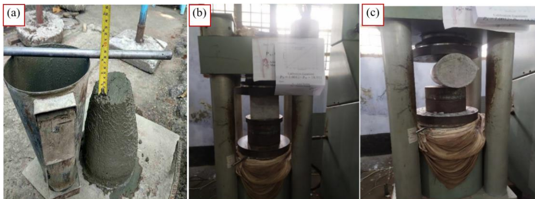
Figure 2. Experimental setup (a) slump test (b) compressive strength test (c) splitting tensile strength test.
