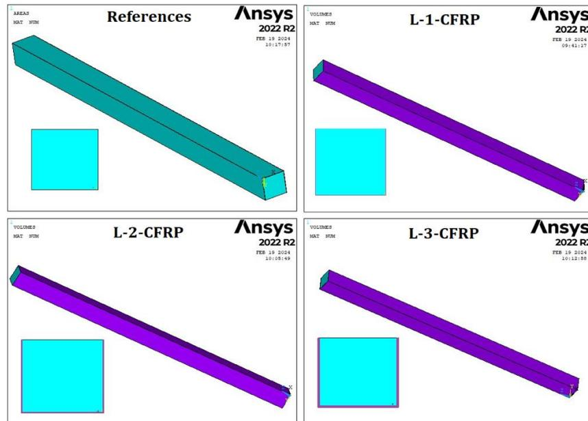
Figure 5. Modeling of beams in a finite element software program.
