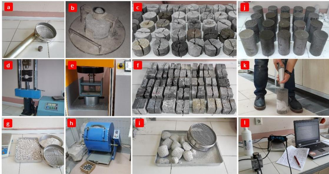
**Figure 5.** Concrete/aggregate tests a) RIHN b) IE test apparatus c) IE specimens after ultimate failure d) BTS<sub>R</sub> e) STSc f) STSc specimens after ultimate failure g) aggregate specimen after 500 revolution h) LA test machine i) and concrete specimen after 500 revolution j) CS<sub>C</sub> and physical test samples k) SHH<sub>C</sub> and l) UPV<sub>C</sub>.
