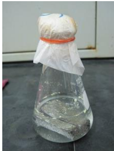
Figure 5. Test piece immersed in the bacterial solution.
