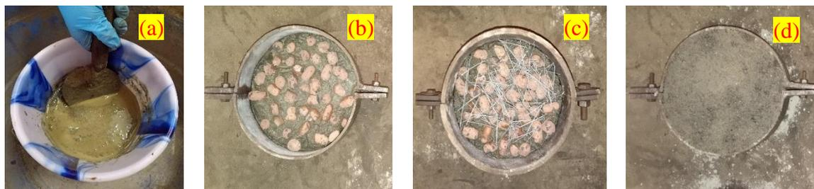
**Figure 8.** Casting procedure for grouted concrete, a) Preparation of grout, b) filling a layer of LWA, c) filling a layer of SF, and d) filling of grout.
