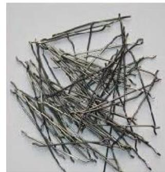
**Figure 4.** Steel fibers.
