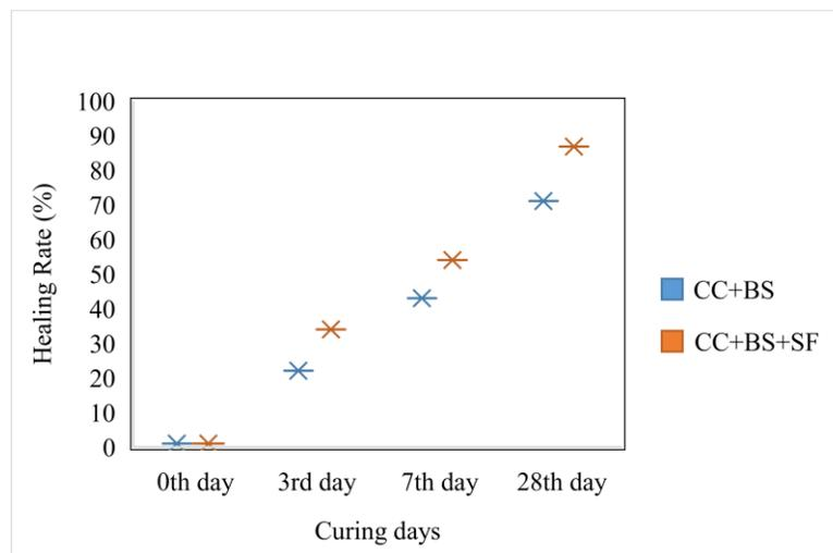
Figure 16. Crack healing % of mix CC+BS and CC+BS+SF.
