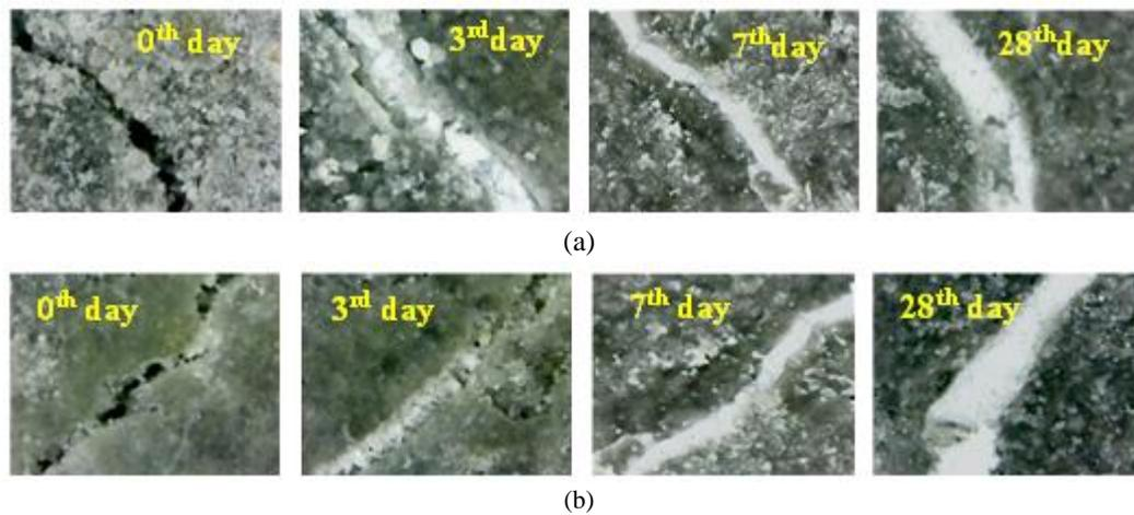
Figure 15. (a) Crack healing of mix CC+BS, and (b) Crack healing of mix CC+BS+SF.
