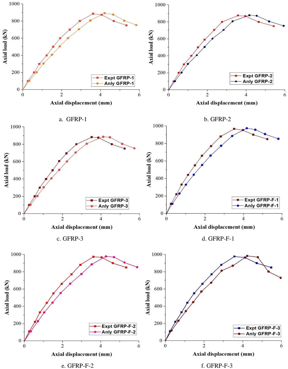
Figure 8. Axial load Vs Axial displacement responses for GFRP RC columns.
