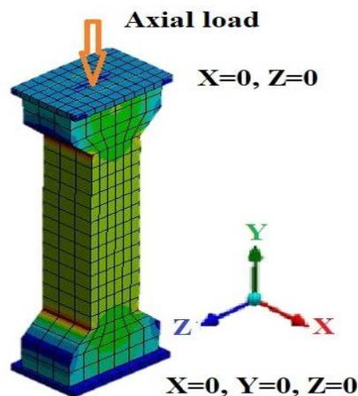
Figure 6. Loading condition of the column.
