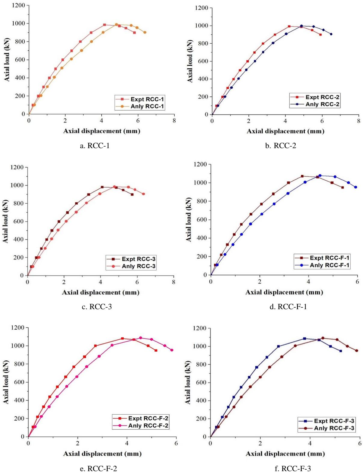
Figure 7. Axial load Vs Axial displacement responses for RC columns.
