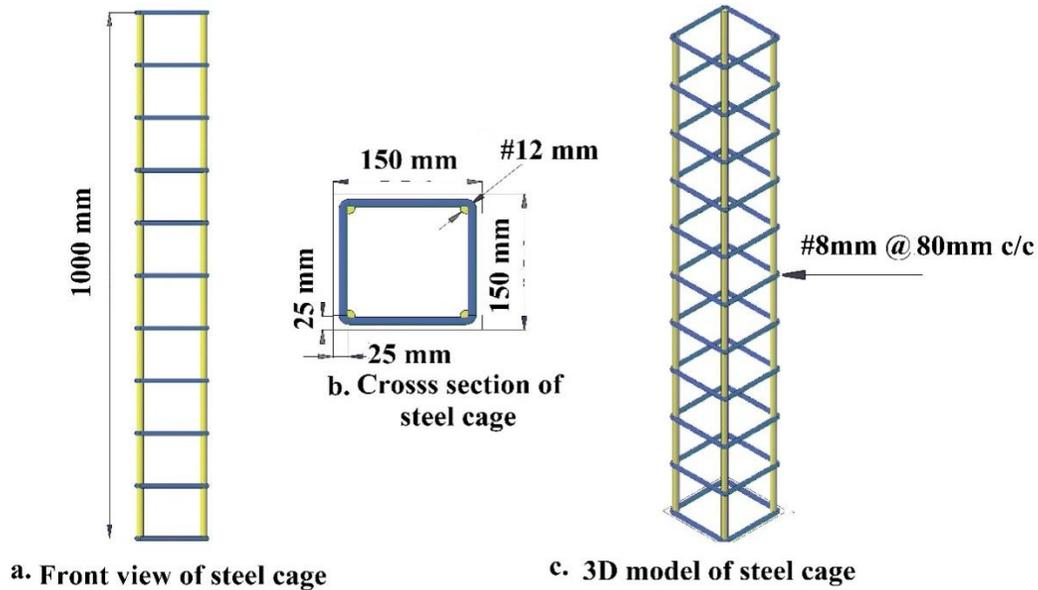
Figure 2. Geometry properties of columns.
