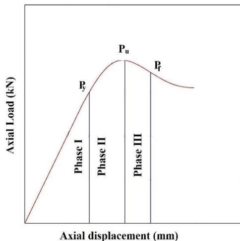
Figure 10. Axial load Vs displacement curve.
