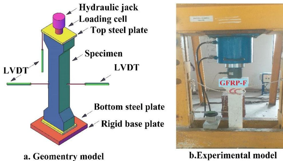
Figure 3. Column setup for testing.
