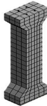
Figure 5. Mesh of high strength concrete column.
