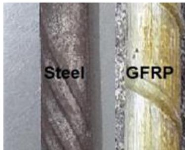
Figure 1. Steel and GFRP bar.
