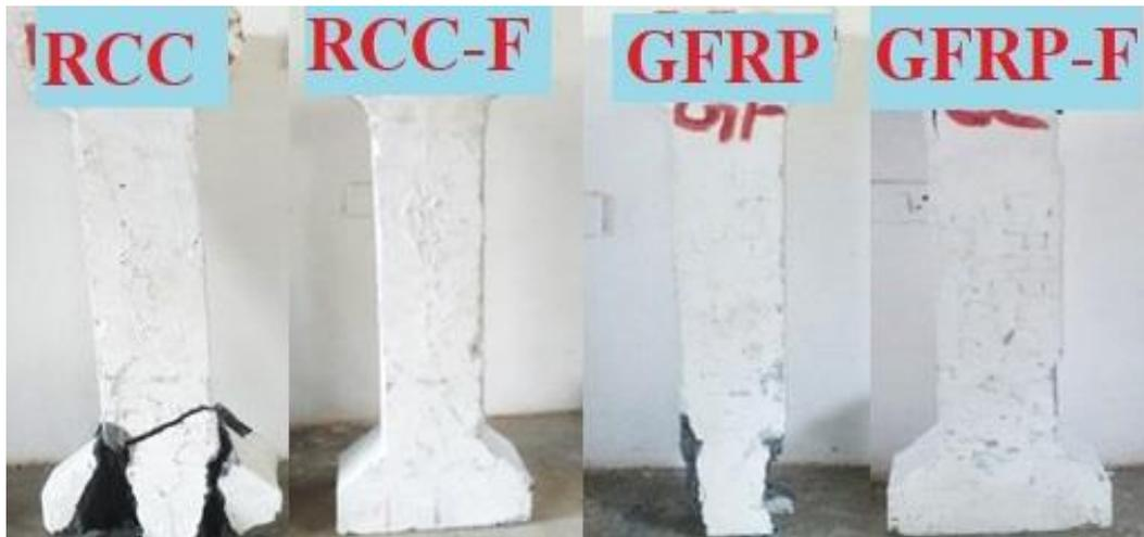
Figure 9. Mode of failure in all columns.
