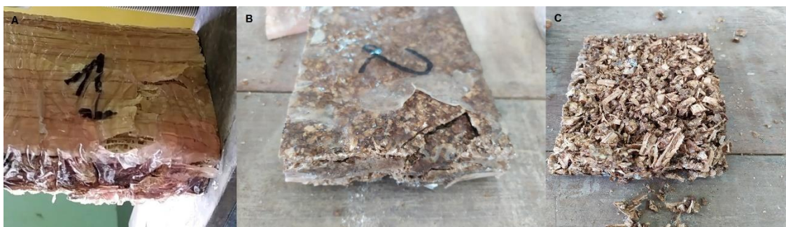
Figure 5. Image of the fracture plane of prototype I (A), II (B) and III (C).
