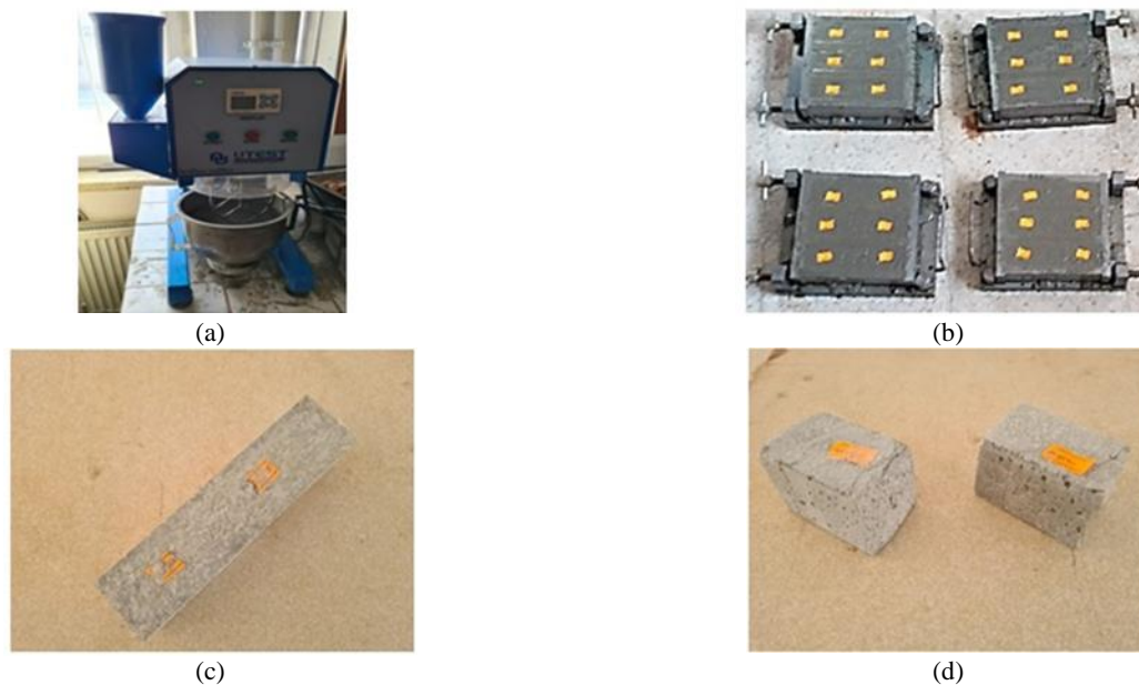
Figure 5. The pictures of the production (a. mixer, b. produced samples, c. cured sample, d. specimens subjected to compressive test).
