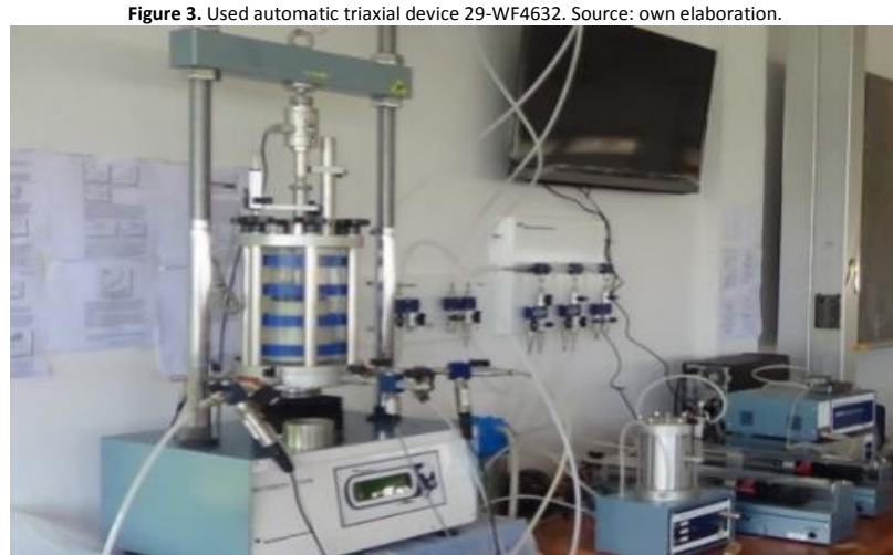
Figure 3. Used automatic triaxial device 29-WF4632. Source: own elaboration.
