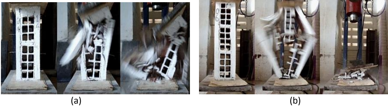
Figure 3. Rupture of the (a) 2 block prisms and (b) 3 block prisms with a coating of 3.0 cm and a mix ratio of 1:2:9 (Source: Self-elaboration, 2016).
