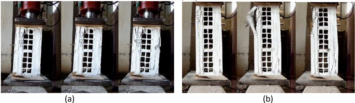
Figure 5. Rupture of the 2 block prisms with a coating of 3.0 cm and a mix ratio of 1:1:6 reinforced with a POP mesh of 10x10 cm and 4.2 mm of diameter (Source: Self-elaboration, 2016).
