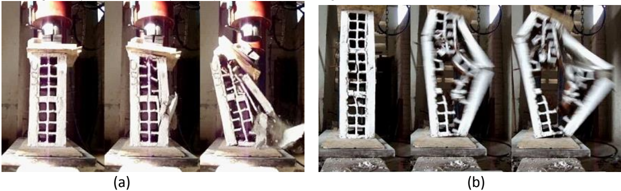
Figure 4. Rupture of the (a) 2 block prisms and (b) 3 block prisms with a coating of 3.0 cm and a mix ratio of 1:1:6 (Source: Self-elaboration, 2016).
