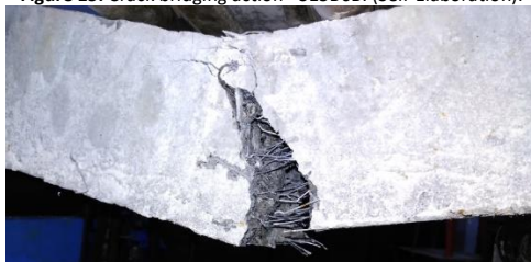
Figure 15. Crack bridging action - S15B6B. (Self-Elaboration).
