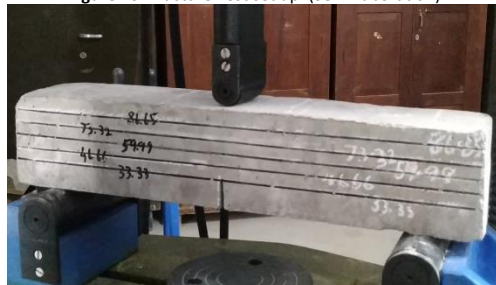
Figure 21. Crack propagation from the notch - CO mix (Grayscale image). (Self-Elaboration).
