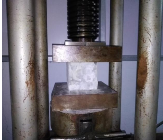
Figure 3. Compressive strength – setup. (Self-Elaboration).
