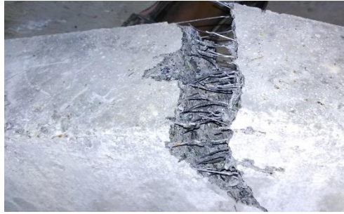
Figure 16. Pullout of steel fibers at the fractured section. (Self-Elaboration).
