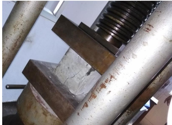
Figure 3. Failed specimen under compression - S15B6B. (Self-Elaboration).
