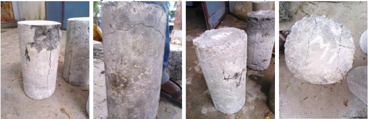
Figure 6. Failed specimens under compressive stress strain. (Self-Elaboration).
