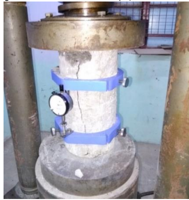
Figure 6. Failed specimens under compressive stress strain. (Self-Elaboration).
