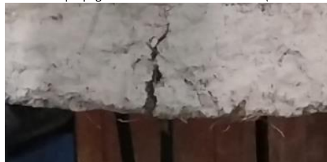
Figure 23. Crack propagation from the notch - S15B6B. (Self-Elaboration).
