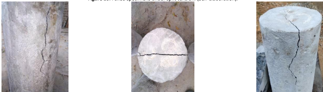
Figure 10. Failed specimens under split tension. (Self-Elaboration).
