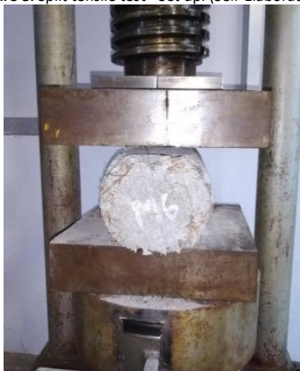
Figure 8. Split tensile test - Set up. (Self-Elaboration).
