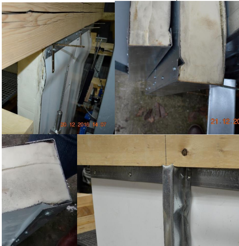
Figure 7. Main deformations obtained in tests. Images in order test 1, test 2 in first file and test 3 and 4 in second file. Source: Self-Elaborated. UPM Structure Laboratory.
