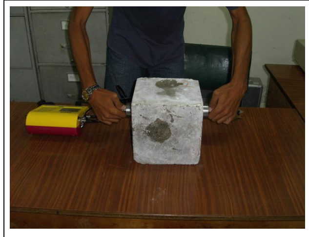
Figure 1. Ultrasonic pulse velocity measuring in the concrete probes. Source: own elaboration, 2010.
