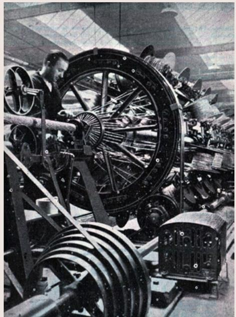
**Figure 6:** Stranding machine made by the German industry Siemens. Unknown author. Source: *Técnica y Cultura* N° 9, July 1938, p. 26.
